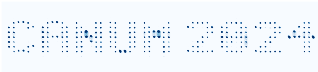
FIGURE 1 – BEC "printer" : each of the columns of this image is a single measurement (absorption image) of the momentum distribution of a Bose-Einstein condensate (BEC) in an optical lattice, taken after optimal preparation of an equal-weight momentum superposition of momentum states from -3 to +3 lattice momentum units.
