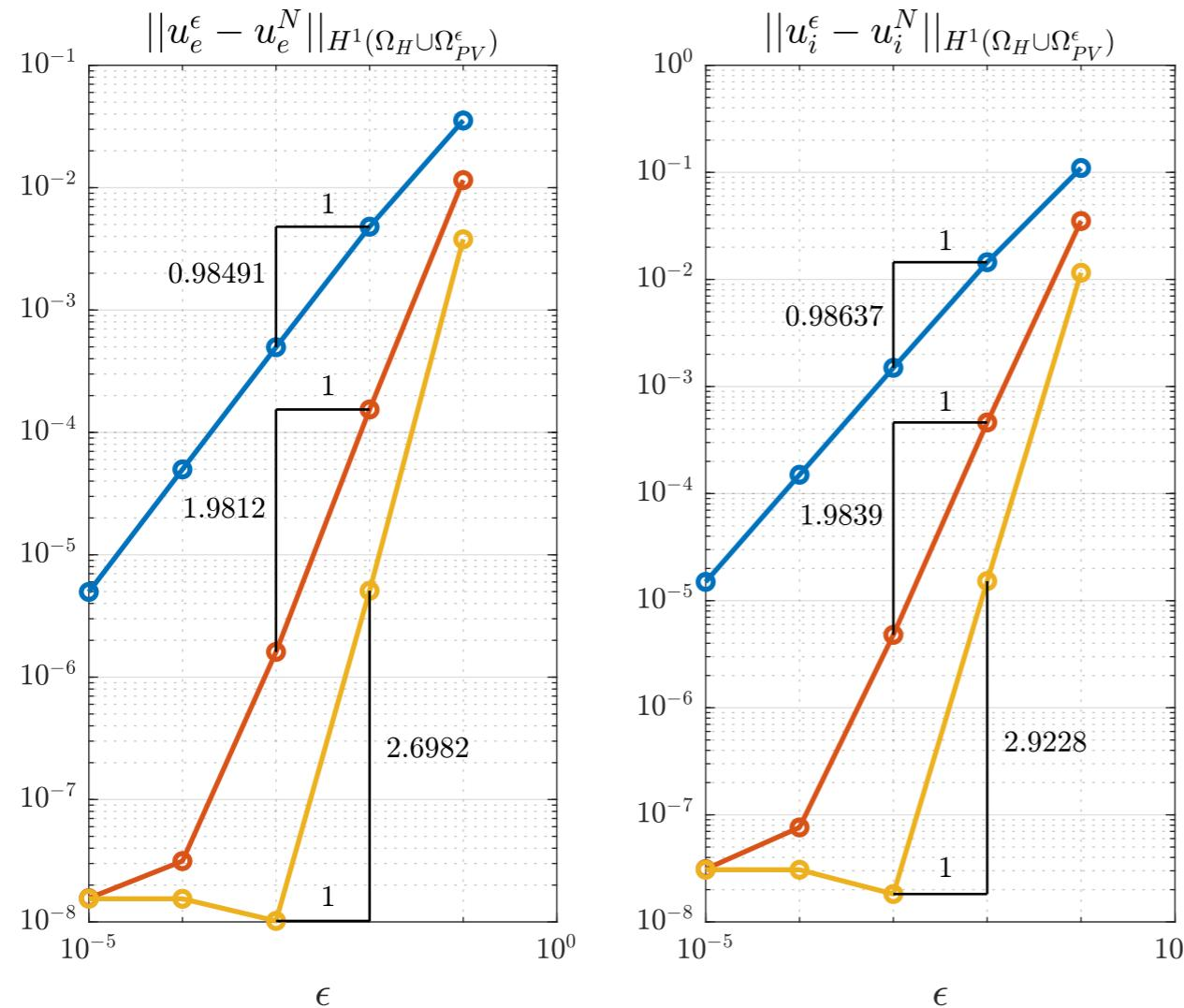
Numerical validation through convergence tests for the zero and first orders
